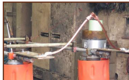
Current Cycle Test per IEEE 837-2014
