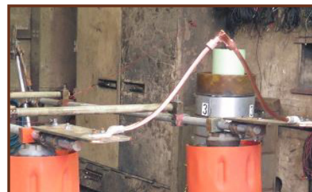
Current Cycle Test per IEEE 837-2014
